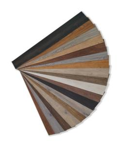
design you want to create, and a "mind's eye" view of your finished project. These Loose Lay Planks are designed to be installed, using minimal or no adhesive and leaving a 5mm expansion gap around the edges. This allows the floor to expand and contract with weather. As such they are recommended for use in areas that maintain a fairly constant temperature and generally remain between 12°C and 29°C on a daily basis.
